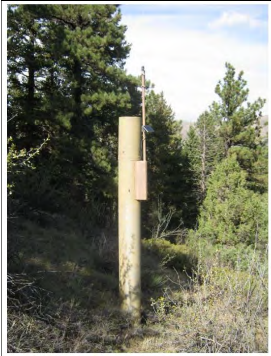
Photo of the Slaughterhouse rain gauge instrument located within the James Creek watershed.
